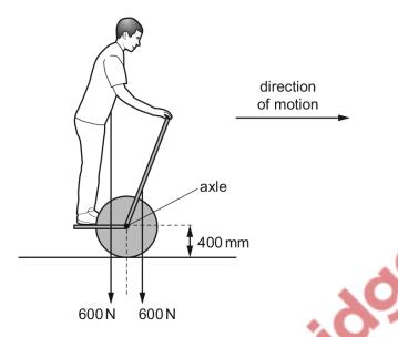
The vehicle has two wheels on one axle. The passenger stands on a platform between the wheels.
