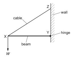
The beam supports a weight W at point X. The forces in the cable and the beam are  $F_{\mathbb{C}}$  and  $F_{\mathbb{B}}$  respectively.
