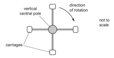
A motor rotates the central pole about its axis. This results in the four carriages each moving along a circular path.
