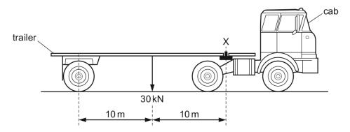
What is the upward force exerted at X by the cab on the trailer?
